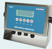
4850 Battery Powered Bluetooth Weight Indicator Drives Up To Eight 350 Ω Load Cells Remote Display, Peak Hold, Checkweighing, Self-Diagnostics
