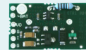
WTS-BC1 Telemetry Charger Module Lithium battery charger module Compatible with both WTS and BTS
