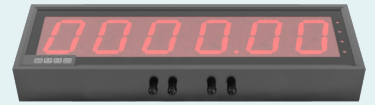
WTS-LD2 Wireless Large LED Display Large Screen with 6-digit 4 in (102 mm) LED display
