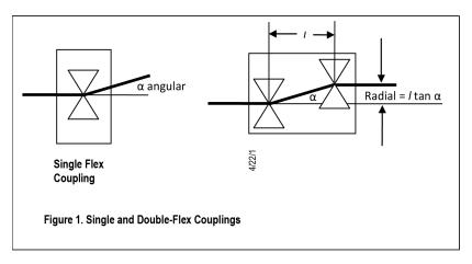
Some available styles of coupling are flexible disk couplings which are desirable for torque measurement because of their high torsional rigidity and zero backlash. Torsional rigidity allows for fast dynamic response and low wind-up. A less rigid coupling will mechanically dampen the signal, possibly reducing or eliminating the ability to measure transient events. Another desirable quality of flexible disk couplings is they can be balanced for high RPM operation.
