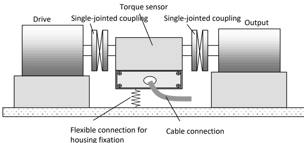
In this case, with both single-jointed couplings, the torque sensor forms a double-jointed coupling. A single-jointed coupling can only balance axial and angular misalignments.
