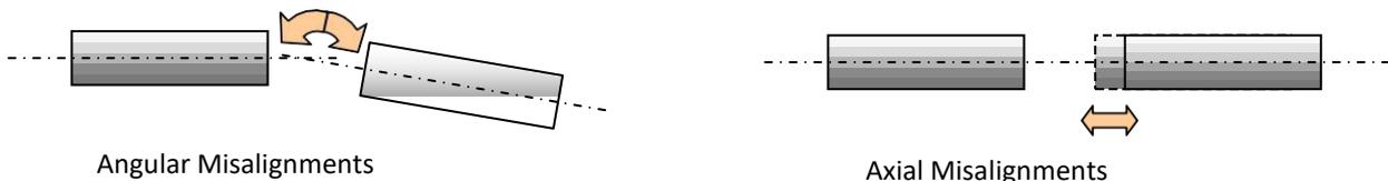
**Note:** Radial misalignments are only possible in the combination of single-jointed coupling - torque sensor (as adapter) - single-jointed coupling. Thus, with both single-jointed couplings the torque sensor forms a double-jointed coupling.
