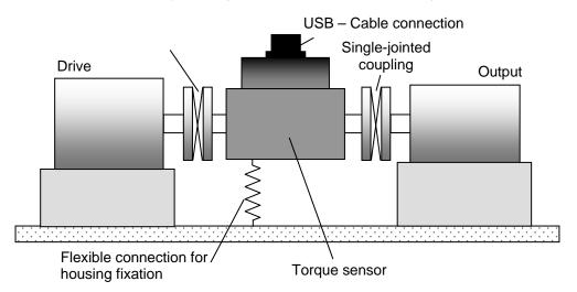
In this case, with both single-jointed couplings, the torque sensor forms a double-jointed coupling. A single-jointed coupling can only balance axial and angular misalignments.
