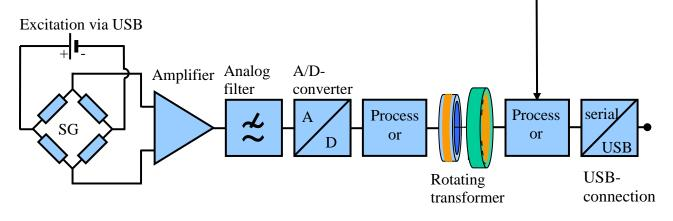
Block diagram for sensor with integrated electronics.
