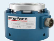
1216 2-Axis Axial Torsion Flange Mount Load Cell Force: 250 lbf to 2K lbf Torque: 125 lbf-in to 1K lbf-in Force: 1.11 to 8.9 kN Torque: 14.1 Nm to 113 Nm Fz, Mz
