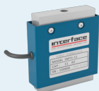
SMT Overload Protected S-Type 1.1 lbf to 450 lbf 5 N to 2000 N 500% +1,000% FS Safe Overload
