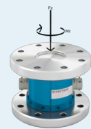
5600 2-Axis Axial Torsion Force: 6K lbf to 180K lbf Torque: 5K lbf-in to 300 lbf-in Force: 27 kN to 800 kN Torque: 560 Nm to 33K Nm Fz, Mz
