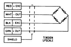
Wiring Code Complies with ISA S37.8 "Specification and Tests for Strain Gage Force Transducers" and SMA Load Cell Terminology.
