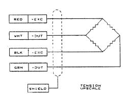
Wiring Code Complies with ISA S37.8 "Specification and Tests for Strain Gage Force Transducers" and SMA Load Cell Terminology.
