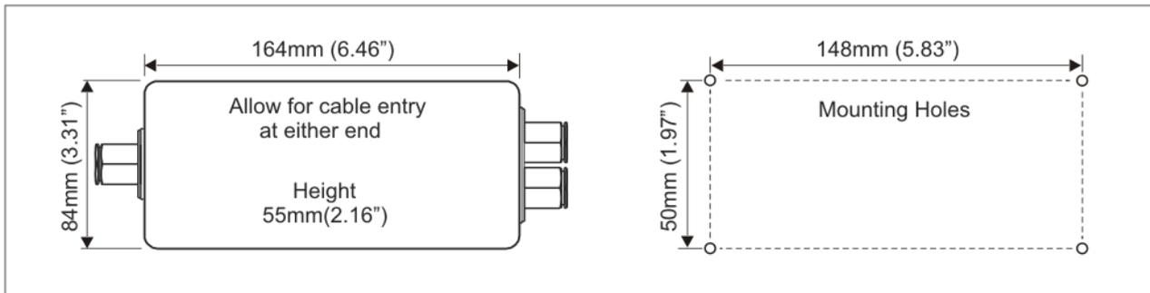
The 4 screws for the lid are captive and must be tightened to maintain the seal.
