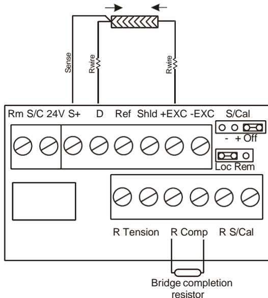
3-wire connection compensates for the resistance of the cable cores.
