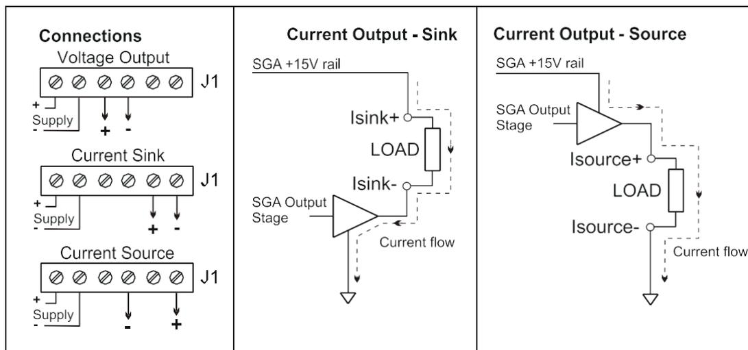
In 'Sink' mode the positive end of the load is connected to the internal +15V supply on the SGA and the negative end is connected to the SGA output. The current through the load is 'sunk' by the SGA towards ground (0V). N.B. In this mode neither connection to the output load is electrically common to the load cell.
