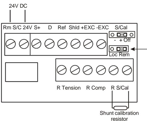
The RSC can be supplied when ordering an SGA or SGA-D or ordered separately for retro-fitting to existing SGAs.
