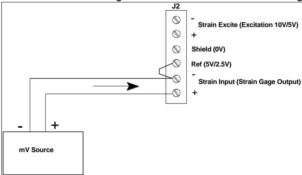
1. The 'Ref (5V/2.5V)' should be connected to 'Strain Input-' and the mV source applied between 'Strain Input+' & 'Strain Input-'
