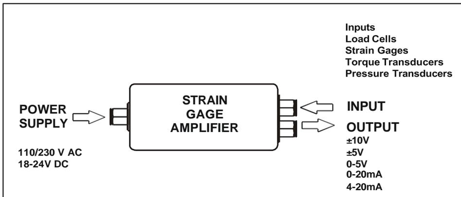
Offered in two versions, the SGA for 110/230V AC or 18-24V DC operation and the SGA-D which is DC powered only.
