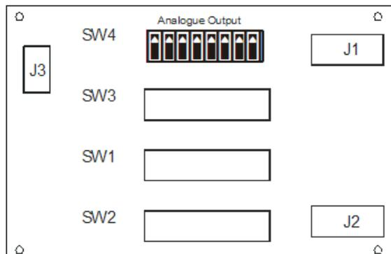
Use switch 4 to select the required output and, if required, the low pass filter and 5V Excitation. (See Tables 3.1 and 3.2)
