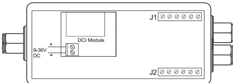
The power supply should be capable of supplying at least 1A for 12V installations and 0.5A for 24V.
