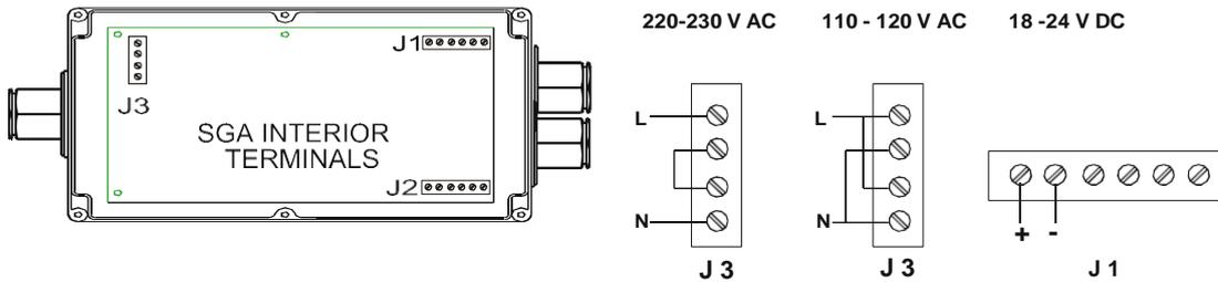
Standard mains 2 or 3 core cable PVC sheathed (unshielded) cable will suffice for the power.
