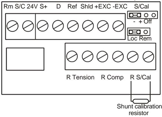
**Remote Shunt Calibration (RSC)**
