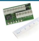
The SGABCM is a retro-fit PCB which facilitates connecting a half or quarter-bridge strain gauge to the SGA Load Cell conditioner.
