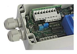
Screw the SGABCM Module into the normal load cell connector J2
