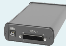
BSC4D Multi-Channel Bridge Amplifier and PC Interface Module 4-Channel Capability
