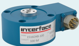
1516 2-Axial Torsion Load Cell 100 lbf, 50 lbf-in 444.9 N to 5.6 Nm
