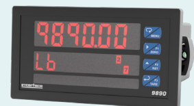
9890 Strain Gage, Load Cell, & mV/V Indicator ±15, ±25, ±150, ±250 mV Bipolar Input Ranges Powers up to 12 x 350 ohm Sensors
