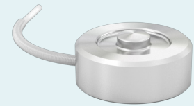
LBM Compression Load Button Load Cell 25 lbf to 50K lbf 0.11 kN to 222.4 kN
