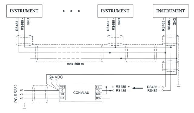
If the RS485 network exceeds 100 meters in length or a baud-rate over 9600 is used, two terminating resistors are needed at the ends of the network: close the two jumpers indicated in the picture on the furthest instruments. If there are different instruments or converters, refer to the specific manuals to determine whether it is necessary to connect the above-mentioned resistors.
