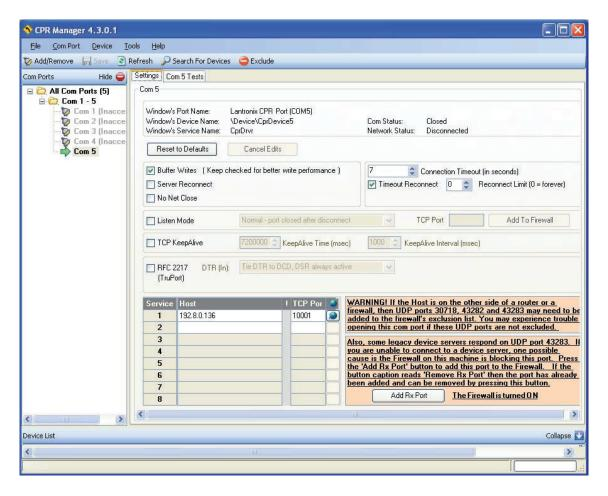
Use the just created virtual COM port to communicate with the instrument, using the protocol selected on it.
