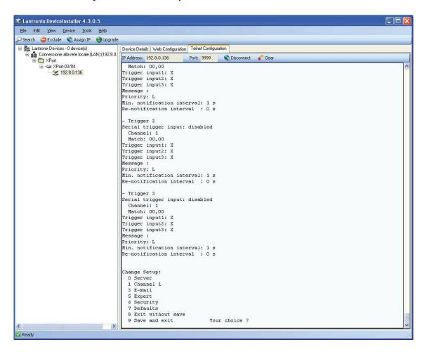
Press 0 to change server settings: change only the 4 fields of IP address and confirm the other parameters by pressing Enter. Set a static IP address.
