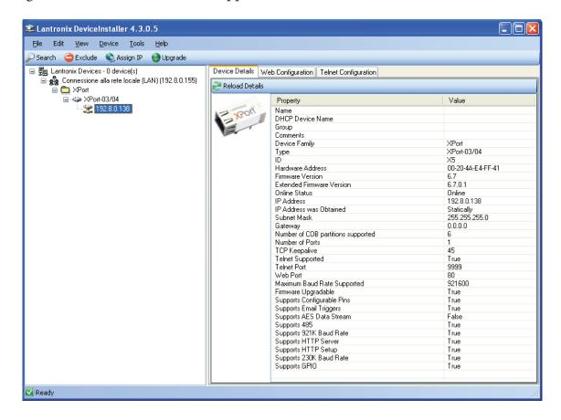
Select the found device and click on the Telnet Configuration tab. Click on Connect, and then press Enter on keyboard.
