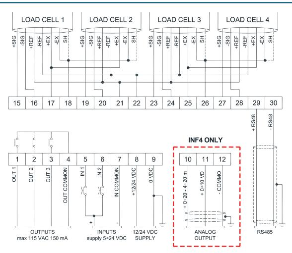
In case of difficulty connecting all the reference wires of the installed load cells, simply connect those of the load cell located at the average distance from the instrument. The reference wires not used must be individually isolated.
