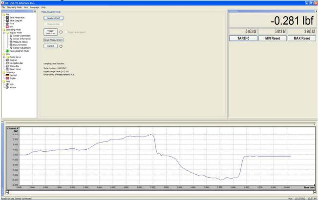
In the **'Meas**./**Diagram Mode'** the digital displays of the physical variables and the diagram can be activated. Only the displays which were check-marked in 'Measure Adjust.  $\rightarrow$  Measured variable  $\rightarrow$  Type' are active.
