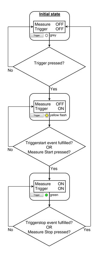
In the previous signal flowchart, the general course of measurement by means of a triggering is described. The activation button **'Trigger'** can be found in the **'Meas./Diagram Mode'** under **'Measure Stop'**. The software triggering consists of two events which are adjustable according the requirements as follows:
