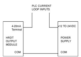
Since the 4-20mA output is configured to sink 4-20mA, a provision must be made to power the loop. This is usually accomplished by using power available at the data acquisition equipment, a PLC current input card for example. Power from the 24 V supply terminals on the Output Module may also be used.
