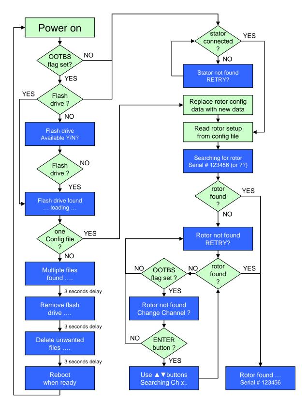
The output module is designed to accept a standard USB flash drive containing factory calibration and setup information.
