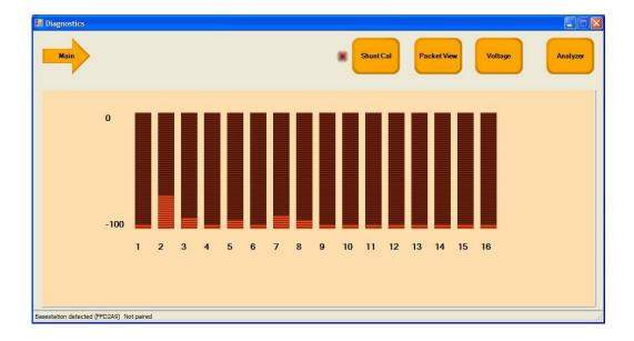
The spectrum analyzer page is helpful for determining radio traffic on the various channels.
