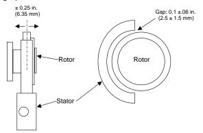
The mounting plate on the stator module can be removed if a custom-mounting bracket is being used. A shorter stator to output module cable can be used if excess cable is a problem.
