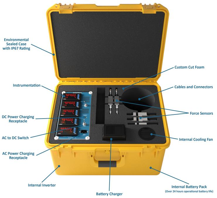
**Custom Portable Battery Powered Force Sensor and Instrumentation Case**
