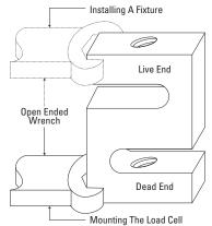
because the mating process between the product you are measuring, and the load cell determines the sensors ability to perform accurate readings. Always make sure to follow the mounting instructions that come with the load cell to ensure accuracy.
