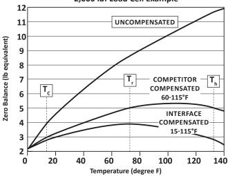
Every Interface Load Cell is Compensated Cold and Hot
