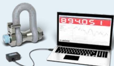
The WTS Wireless Crosby Load Shackle measures lifting and tension forces, transmitting data to the WTS-BS-4 Base Station via secure long-range telemetry. Connected to a PC, the base station streams data into Log100 software for real-time logging and visualization of up to 100 channels with customizable layouts and browser-based remote monitoring.
