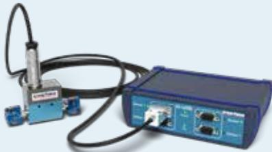
Interface's A T2 Ultra-Precision Shaft-Style Rotary Torque Transducer measures dynamic torque with high accuracy and optional speed/angle sensing. It connects via a Floating-Mount Single-Flex Coupling to ensure torsional stiffness and eliminate misalignment. The SI-USB4 Interface Module then digitizes the analog signals at 16-bit resolution for high-speed data capture on a PC.
