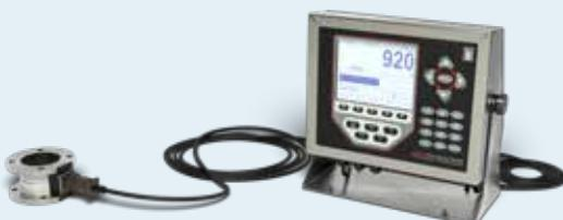
The 5330 Hollow Flange Style Reaction Torque Transducer detects static torque via strain-gage deformation and outputs a signal (mV/V), while the 920i Programmable Weight Indicator and Controller receives that signal, digitizes it at up to 960 Hz, displays multiple channels in real time, and enables calibration, setpoints, and control.
