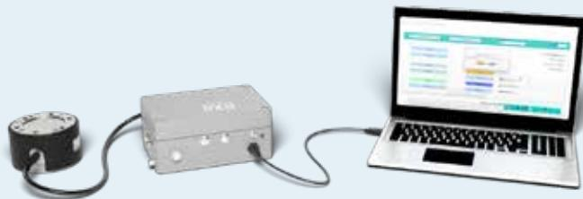
Interface's 6A-Series 6-axis load cell captures forces (Fx, Fy, Fz) and torques (Mx, My, Mz) across six channels, while the BX8-AS BlueDAQ data acquisition system logs, graphs, and outputs all six measurements in real time creating a complete, high-resolution multi-axis measurement solution.
