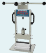
IFVF-2.5K Interface Force Verification Frame 2,500 lbf ± 2.5k lbf Handle Rotation
