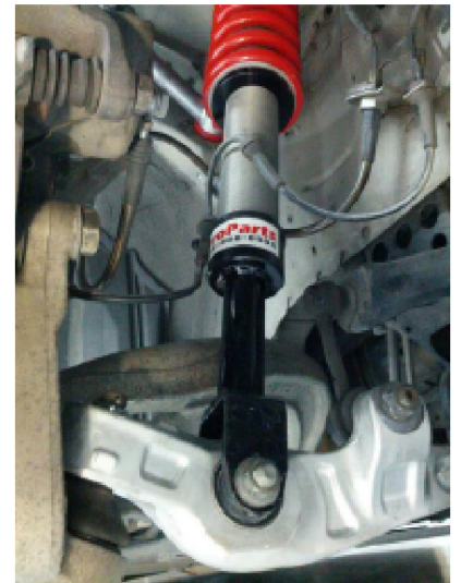
Figure 3. Koni adjustable shock absorber and specifically rated coilover spring.
