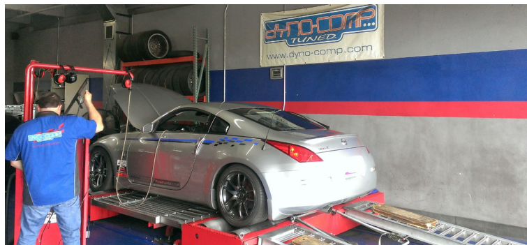
Figure 3. Used to measure the braking force / torque, load cells are integral parts to chassis dynamometers. Nissan 350Z's engine control unit being tuned for 100 octane gasoline
