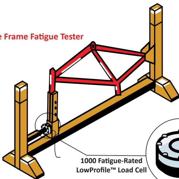
1000 Fatigue-Rated LowProfile™ Load Cell
