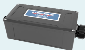
SGA AC/DC Powered Signal Conditioner User selectable analog output ±10V, ±5V, 0-10V, 0-5V, 0-20mA, 4-20mA 110 VAC, 220 VAC OR 18-24 VDC power
