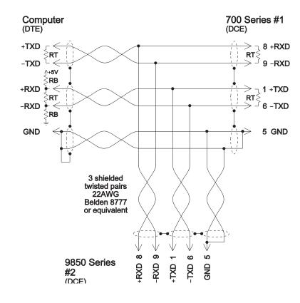
**Termination resistors (RT)** should only be used with high data rates **and** long cable runs. A good rule of thumb is 2000ft at 38400 BAUD. Terminate with  $120\Omega$  at no more than two places; the computer and the 9850 at the furthest end. To use the termination resistors installed in the 9850, see RS485/422 Termination Jumpers in APPENDIX B.
