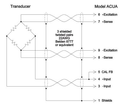
Other than connections shown, isolate shields from other conductors including connector housing.
