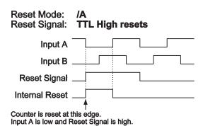
For the following example, Internal Reset is equal to the external Reset signal (inverted) ANDed with Input A (non-inverted) and Input B (inverted). The counter is reset at the leading edge of Internal Reset.
