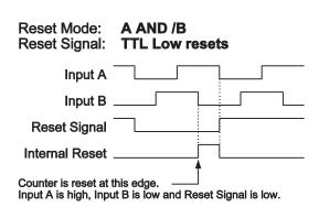
For the example to the right, /B is a poor choice because Input B is low in two places when Reset signal is active. As a result, two reset pulses occur.
