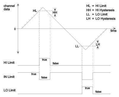
If HI Hysteresis is too small, HI Limit may oscillate true and false when data is near HI Limit value. Similarly, if LO Hysteresis is too small, LO Limit may oscillate true and false when data is near LO Limit value. In *Absolute* mode, the absolute values of data, HI Limit, and LO Limit are used to determine limit violations. For example, a HI Limit violation occurs if data equals -2000 and HI Limit equals +1000.
