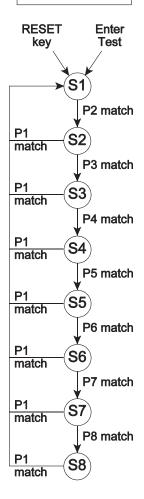
There are eight patterns. For each pattern you define the logic state (or *ignore*) of each logic input, output, and internal Matrix signal. Then, during a Test, patterns are compared to actual signals. Patterns are used in two ways depending on the *State Machine* setting in the *System Options* menu.
