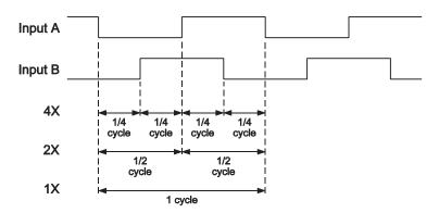
2X and 4X count modes allow finer resolution for displayed data. But, for encoders with many pulses, the finer resolution is not viewable if it is smaller than the Display Resolution. For example, a rotary encoder has 3600 pulses/revolution. For a Full Scale of 360 degrees, the best Display Resolution is 0.050 degrees. The count resolution is determined as shown below.
