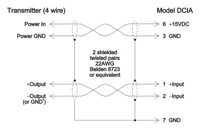
\* If transmitter has single-ended output then connect -Input (pin 2) to GND at transmitter. Do not make this connection at DCIA connector. Instead, run separate wires for Power GND and Output GND as shown in diagram.
