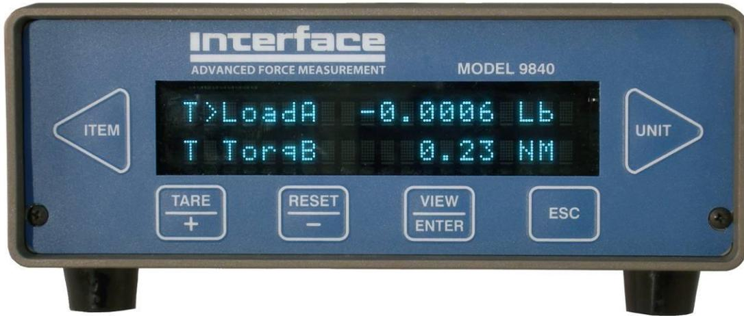
The example above shows that LoadA is -0.0006 Lb. The second line of the display shows TorqB with 0.23 NM. The “T” TEDS<sup>OPT</sup> annunciator indicates presence or non presence of a TEDS<sup>OPT</sup> sensor. If it is on solid, a TEDS<sup>OPT</sup> sensor is attached. If it is blinking a non TEDS<sup>OPT</sup> sensor is attached. The “T” is not displayed when the TEDS<sup>OPT</sup> feature is turned off.
