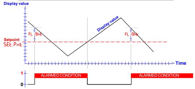
The Setpoint can be placed anywhere you like, in the range \$9999 to +999999 and will include a decimal point in the appropriate position if you have set your display range to have a decimal point.
