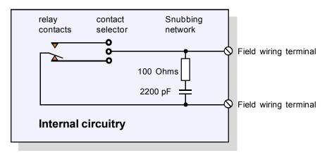
But because you are switching an AC signal, the capacitor is acting as a charge coupler, and your voltmeter is detecting the coupled AC voltage. If you were to use a traditional, lower impedance moving pointer meter, such as an AVO, you would probably not see this effect. The impedance of the capacitor is very high, around 1 500 000 Ohms with 50Hz AC or 1 200 000 Ohms with 60Hz AC.
