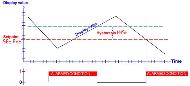
The Setpoint can be placed anywhere you like, in the range 89999 to +999999 and will include a decimal point in the appropriate position if you have set your display range to have a decimal point.
