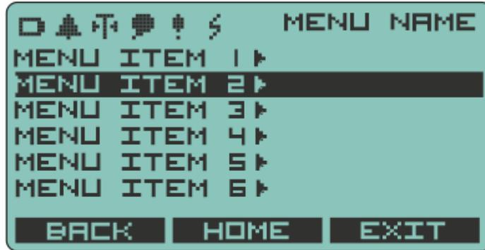
The currently selected menu item is displayed on a dark background and this selection can be changed by using the up and down keys. Pressing OK will select that item and can either:
