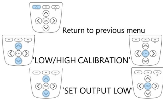
Manually enter the low output required using
