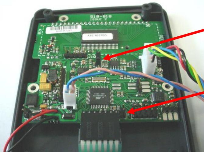
Sensitivity link should be in this position for use with sensors, with sensitivities <+/- 5mV/V
