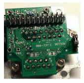
Figure 8 - Location of Rcal direction Jumpers and Rcal resistor.
