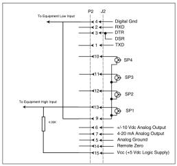
This figure shows that when using an external power to provide power to the set point outputs, the value of the pull-up resistor in ohms should be between SUPPLY VOLTAGE / .01 as the lowest value and SUPPLY VOLTAGE / .001 as the highest. The setpoint common (pin 9) is typically tied to the external supply common pin.
