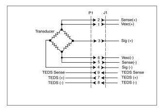
$\label{thm:performance} Figure 3. \ Transducer \ Wiring - NOTE: for optimum performance cable shield should be connected to the instrument chassis.$
