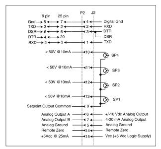
Figure 4. I/O Wiring
