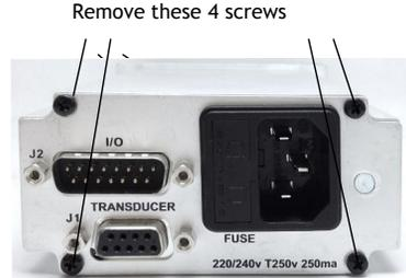
Then gently remove the top cover, to expose the DIP switch and analog output gain adjustment pots
