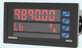
9890 Strain Gage, Load Cell, & mV/V Indicator \pm 15 , \pm 25 , \pm 150 , \pm 250 mV Bipolar Input Ranges Powers up to 12 x 350 ohm Sensors
