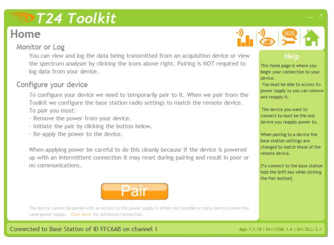
We now have successful communications with the base station so we can now pair with our device or we can select the Spectrum Analyzer mode or Data Provider Monitor mode.
